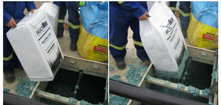
MulchMax can be added without breaking the bales by cutting the bottom of the bag, creating a breather slit in the top of the bag and dropping the entire bale into the mechanically agitated machine without concern of auger jamming.
